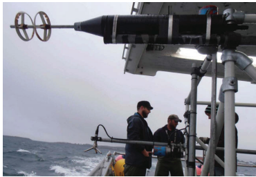
b The velocity sensors: the MAVS (upper left, foreground), and the Vector ADV (middle, background), both cantilevered away from the main body of the pod.
