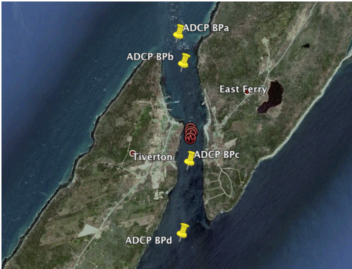
Figure 1: Locations of ADCP deployments in Petit Passage and test case turbine deployment locations in throat of channel (shown with red circular marker)
