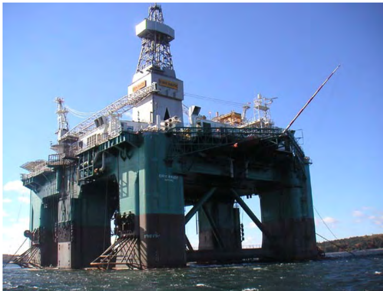
Figure 2.3 Semi-Submersible Eric Raude Floating at Anchor (courtesy of EnCana)
