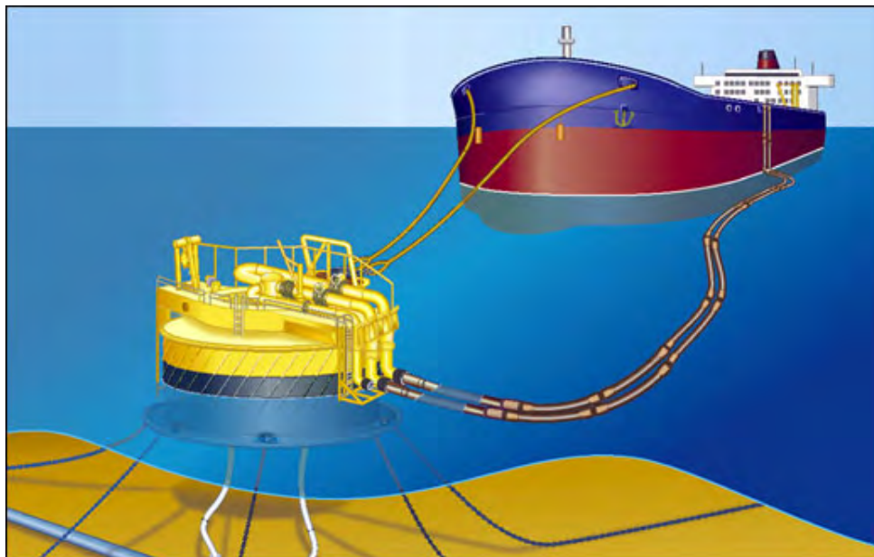
Figure 2.4 Diagram of CALM Buoy and Tanker Filling System (courtesy of IPS Services)
