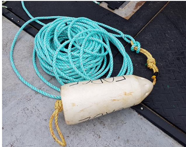
FIGURE 3 TYPICAL SURFACE FLOAT
