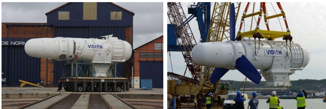
FIGURE 32 - VOITH TURBINE ASSEMBLY AND LAUNCH IN CHERBOURG (SOURCE: ENERGIEDELAMER.EU (LEFT), AFP (RIGHT))
