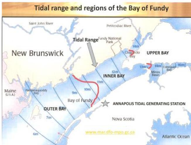
The present approach in Nova Scotia is based upon the conversion of the kinetic energy of flowing water. Tidal stream (or *hydrokinetic*) turbines are analogous to windmills in that they are driven by the forces of flowing water, rather than the 'head' or pressure of water stored behind a dam. Since the new tidal stream devices do not require construction of barrages, they are somewhat less efficient at converting the energy of tidal flows into electricity, but
