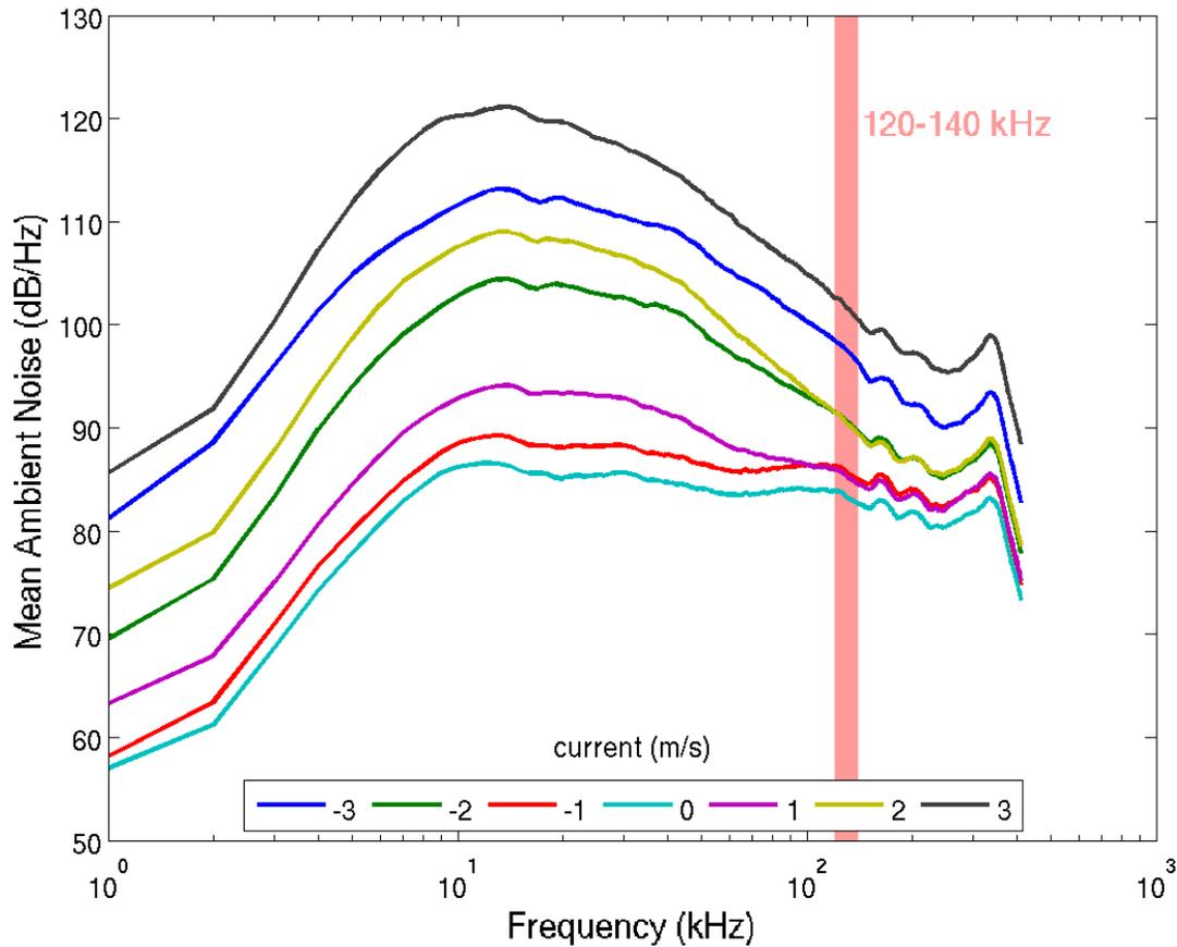
Figure 4.9. *icListenHF* 1239 hydrophone measures of ambient noise (dB/Hz) in Minas Passage, at FORCE monitoring location W1 during 6 June – 2 July 2014, as a function of frequency (kHz) for a range of current speeds ( $\pm 0.1$  m/s) on the ebb (-) and flood (+) tides. The hydrophone was shrouded (20 ppi,  $\frac{1}{2}$  inch foam) and housed on the bottom moored instrument platform. Note that harbour porpoise echolocation click train frequencies are in the range of 120-140 kHz.
