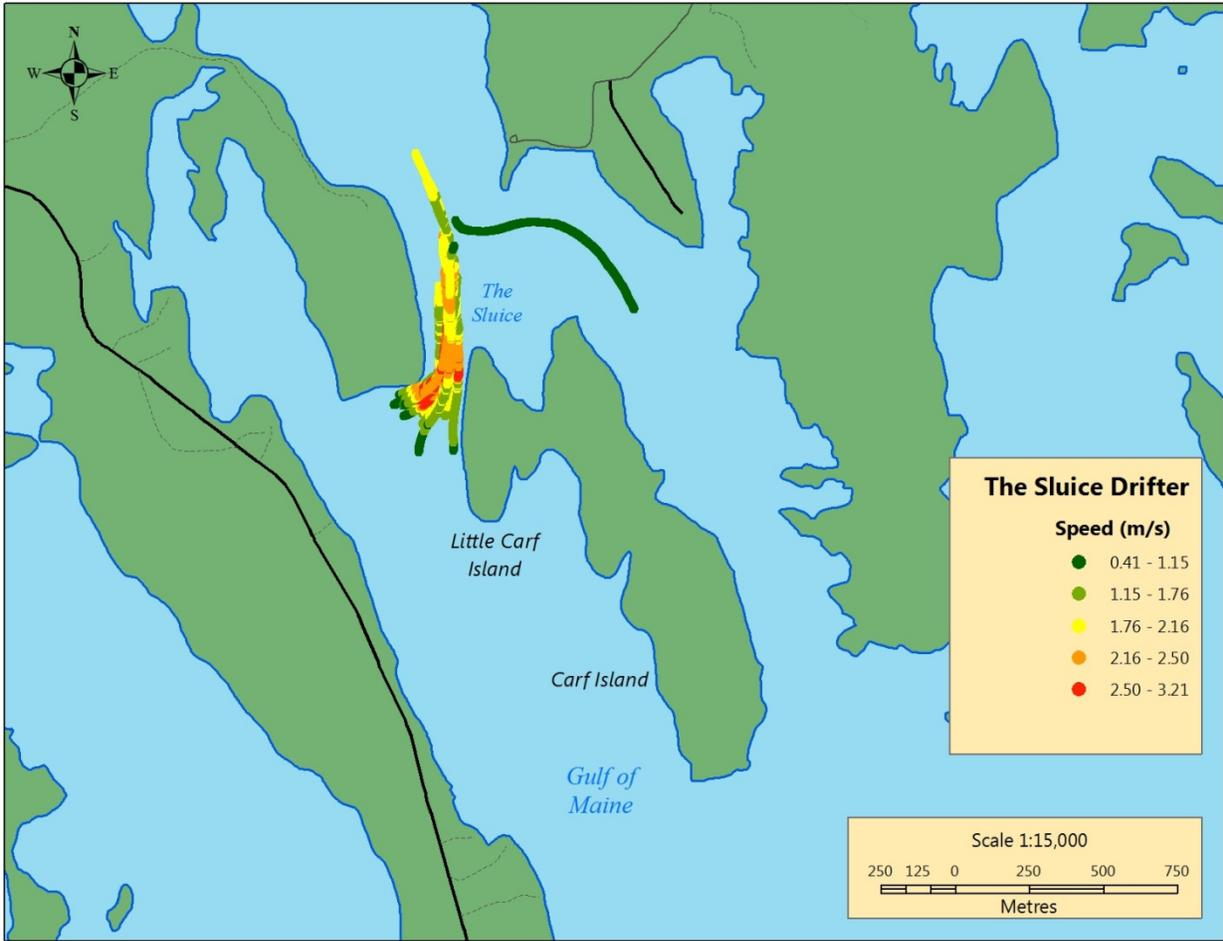
Figure 25 Drifter speed plot of “The Sluice”.
