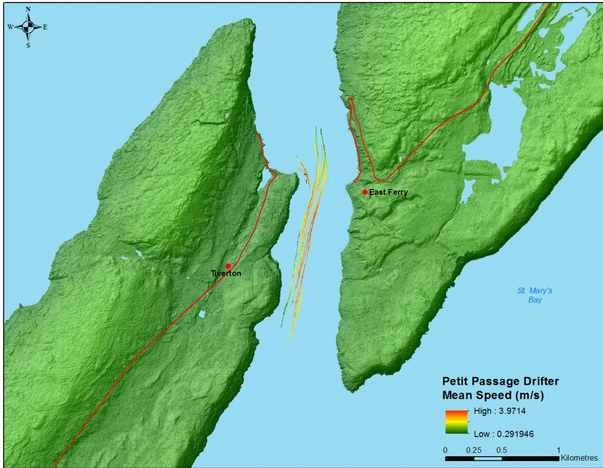
**Figure 27:** Drifter Mean Speed (m/s) in Petit Passage.
