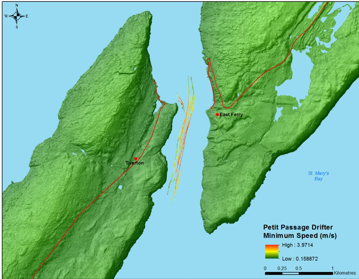
**Figure 29:** Drifter Minimum Speed (m/s) in Petit Passage
