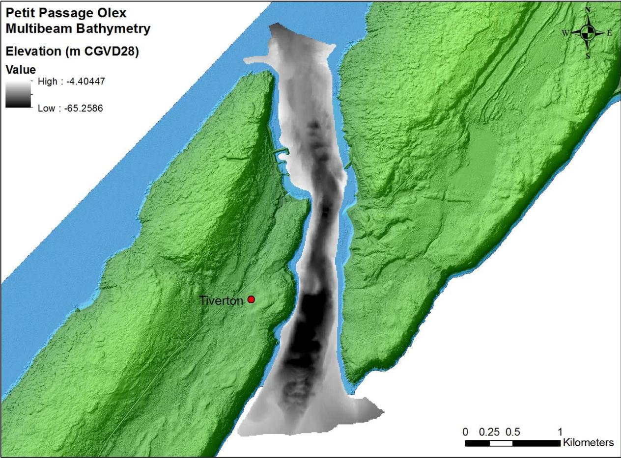
Figure 15: Olex multibeam coverage for Petite Passage.
