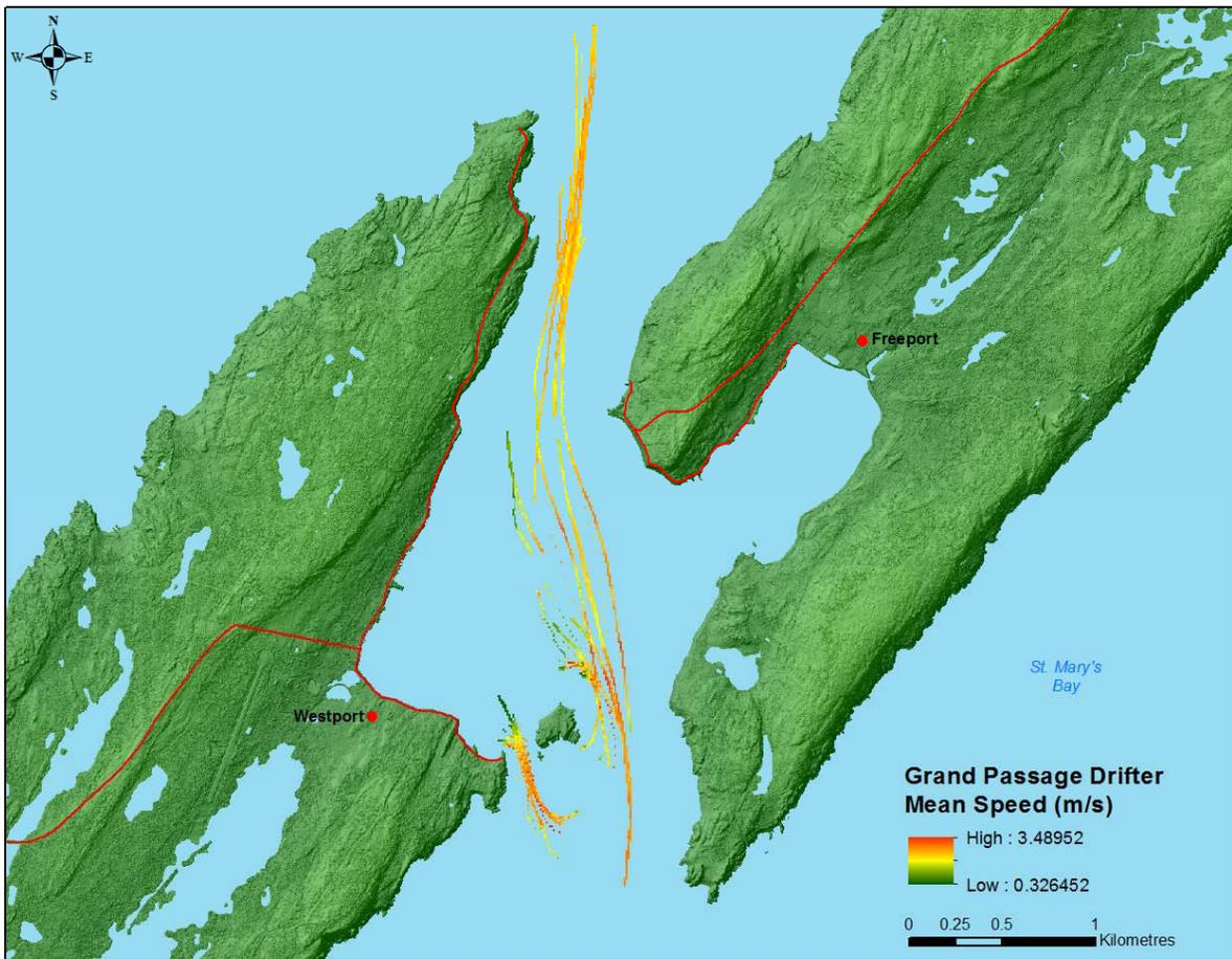
**Figure 24:** Drifter Mean Speed (m/s) in Grand Passage
