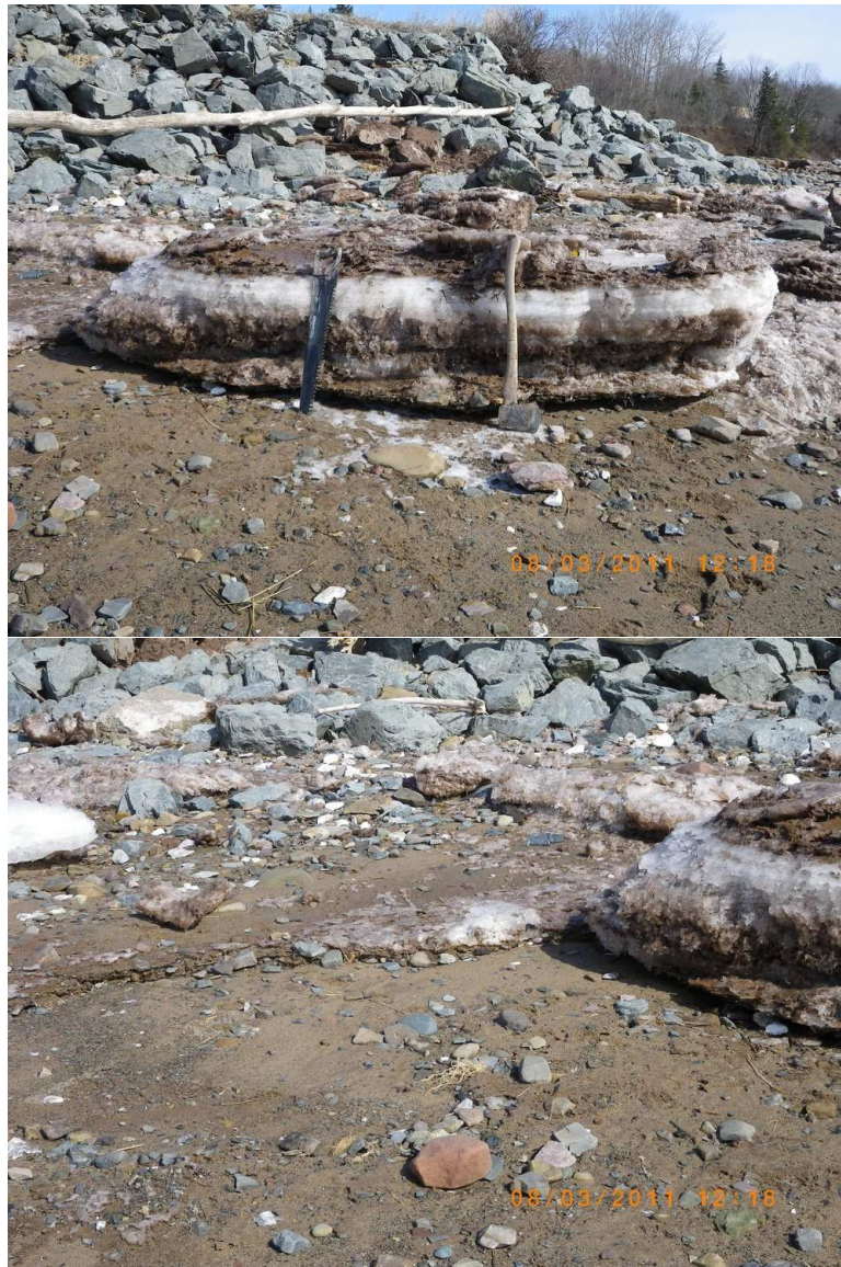
Figure 21: Top: This is ice cake 8 and its position is 45.09810^{\circ} N, 64.18295^{\circ} W. The axe is 83.5 cm long and the axe head has max dimension 18 cm. Most of this ice block is less dense than seawater. But it has settled on frozen gravel and sand which has become attached to the bottom layer. We can see that buoyancy forces seem to have ripped it away from the underlying sand (see bottom photograph) so that the bottom of the ice-block consists of a layer of frozen gravel and sand. Bottom: A thin layer of frozen sediment (sand and gravel) has been removed to the left of ice cake 8. The removed material has dimension and shape consistent with the base of ice cake 8.
