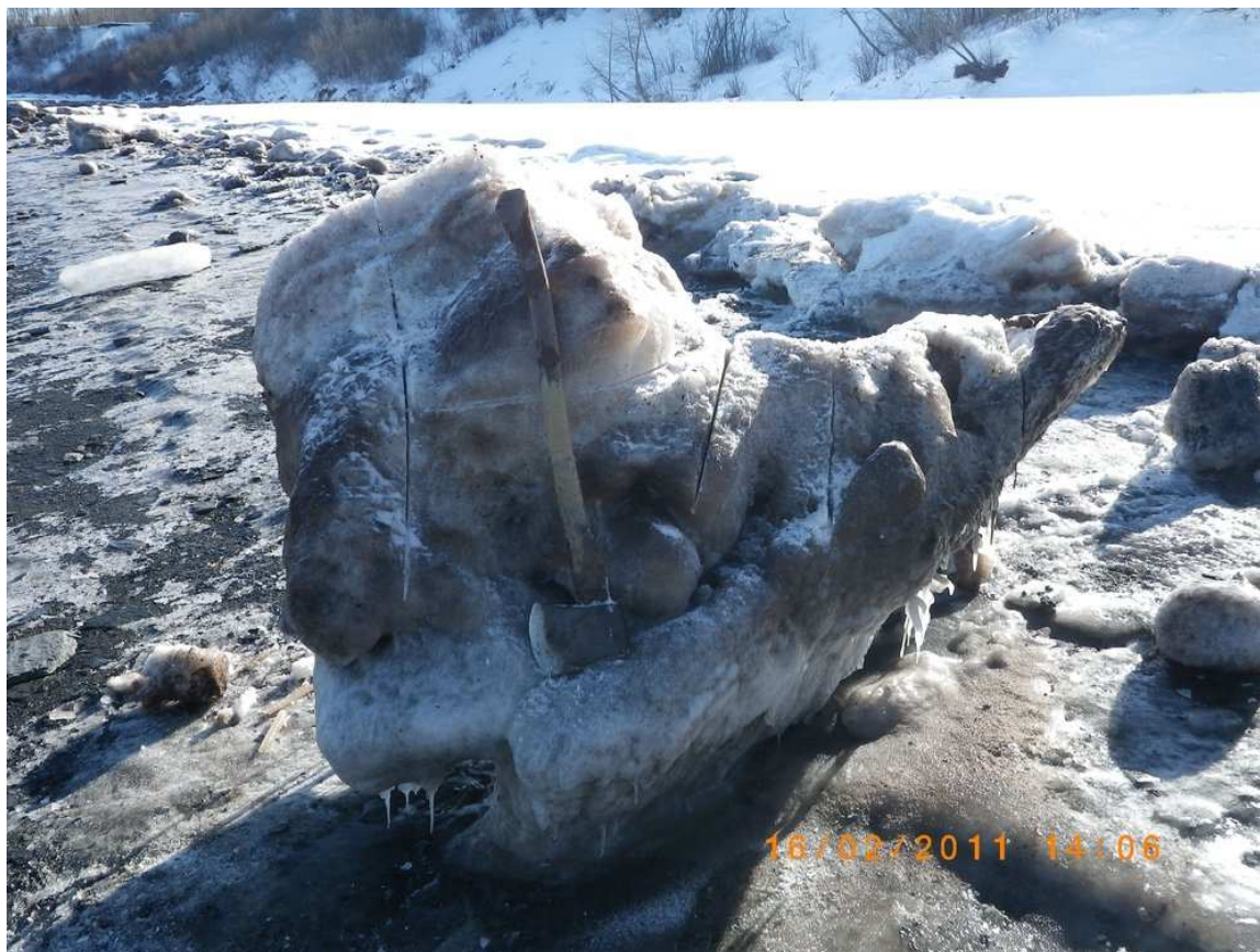
Figure 6: Photograph of ice cake 2 at Blue Beach (45.09667° N, 64.21221° W) on 16 February 2011. Preliminary sampling cuts have been made. The length of the axe is 83.5 m. The ice spear is visible in the upper left corner of the photograph.
