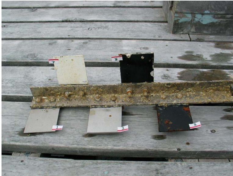
FIGURE 4.4 Biofouling on Materials and Coatings at Race Rocks
