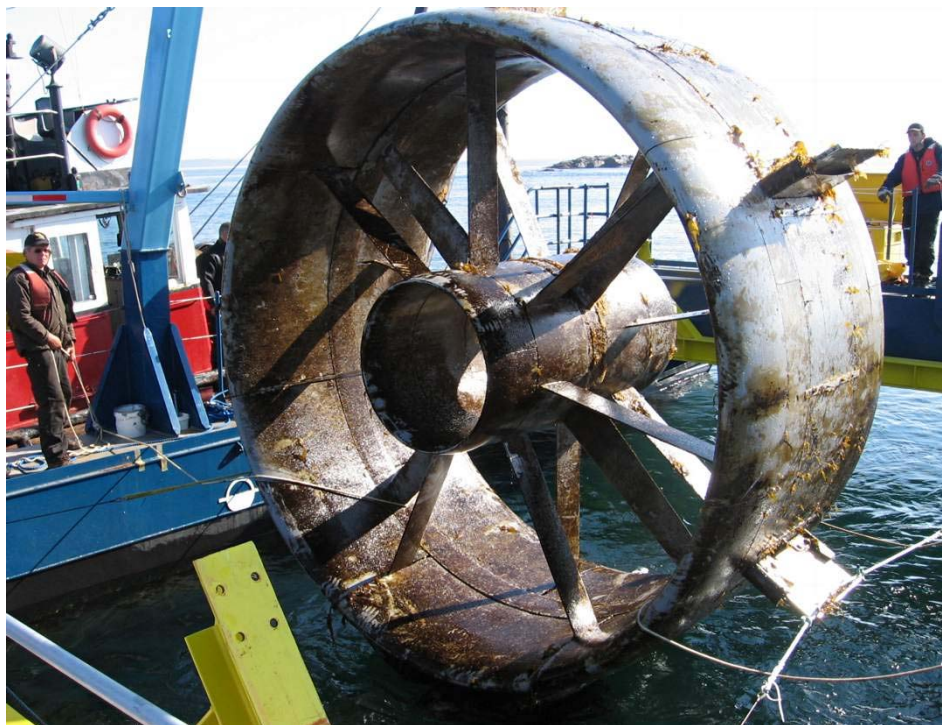
FIGURE 4.6 Turbine Removed After 6 Months of Operation
