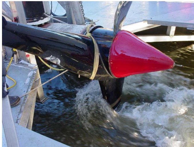
FIGURE 4.2 Verdant Power Initial Turbine Testing
