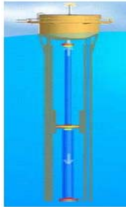
FIGURE 3.11 Buoy-style Point Absorber for Wave Energy Conversion (courtesy Finavera)
