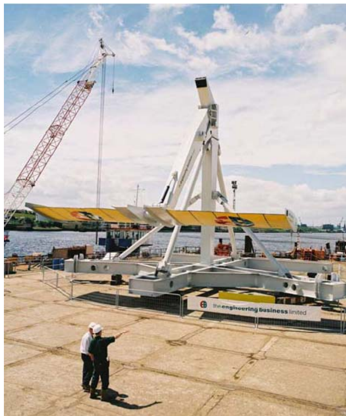
FIGURE 3.5 Image of the Stingray Oscillating Hydrofoil Device (courtesy the Engineering Business)
