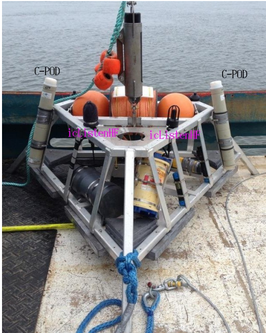
Figure 3: Lander platform with two C-PODs and two icListenHF hydrophones. One icListenHF has a foam shroud over its sensor. Instrument sensors were about 1 m above the seafloor when the lander platform was deployed at the FORCE Crown Lease Area [15].
