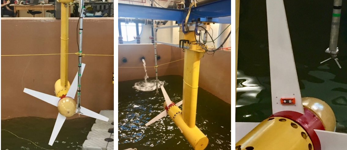
Figure 25: The 4 Fiber Metal Laminate blade hub installed on the turbine and Far right: with accelerometer mounted on the blade.
