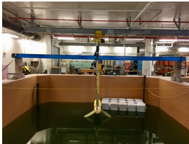
Figure 22: Set up of the three Schottel Hydro SIT250 scaled blades (3 Schottel hub).
