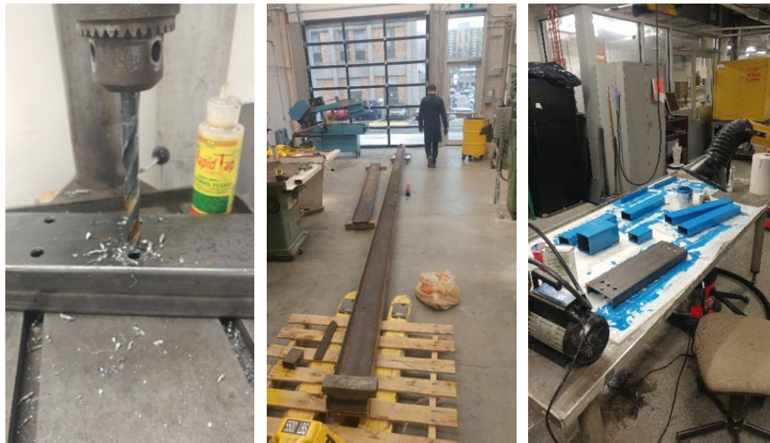
Figure 1: Assembly of turbine support frame
