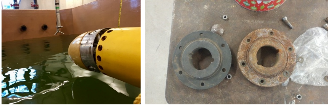
Figure 23: Left: Turbine stopped rotating, nosecone and hub are bent downwards. Right: Rotor collars, damaged collar to the right, new replacement collar to the left.
