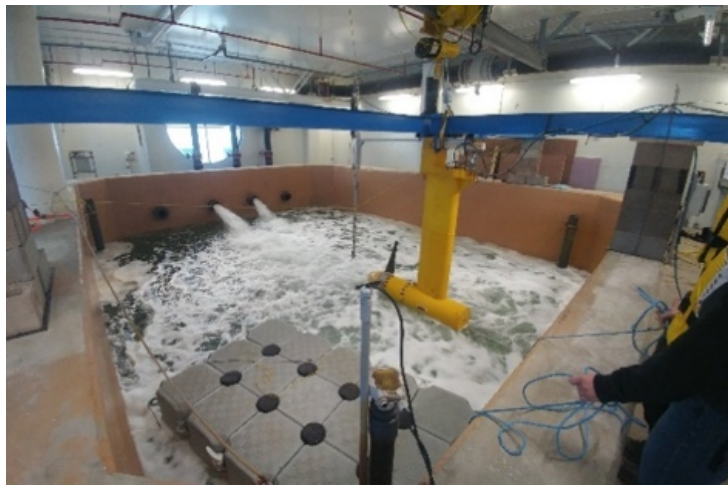
Figure 20: Turbine in tank experimental setup
