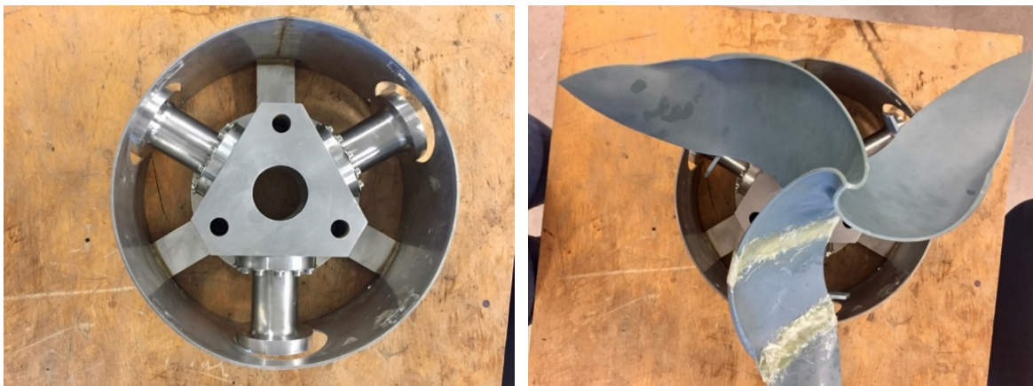
Figure 27: Left: 3 Schottel hub without blades. Right: Ceramic PowerCone on 3 Schottel hub.
