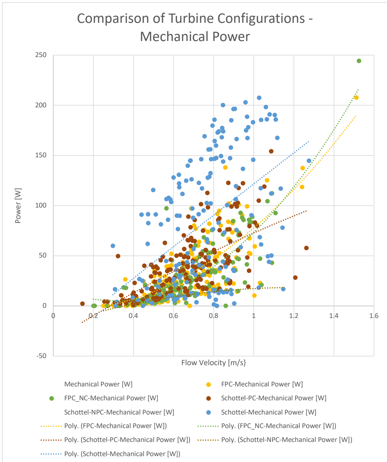
Figure 48 Mechanical Power versus Flow velocity for a number of configurations
