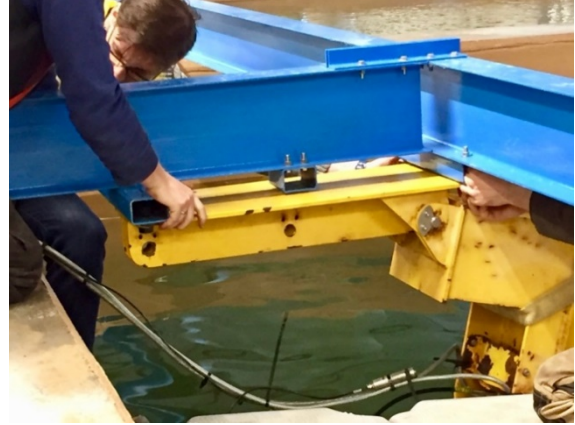
Figure 9 Turbine being attached to frame
