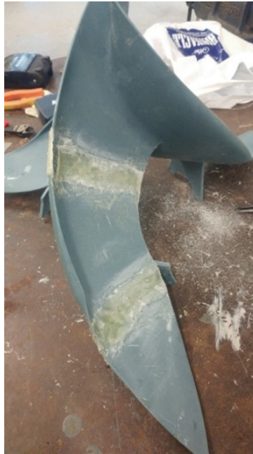
Figure 12: Ceramic PowerCone fixed with epoxy and fiberglass
