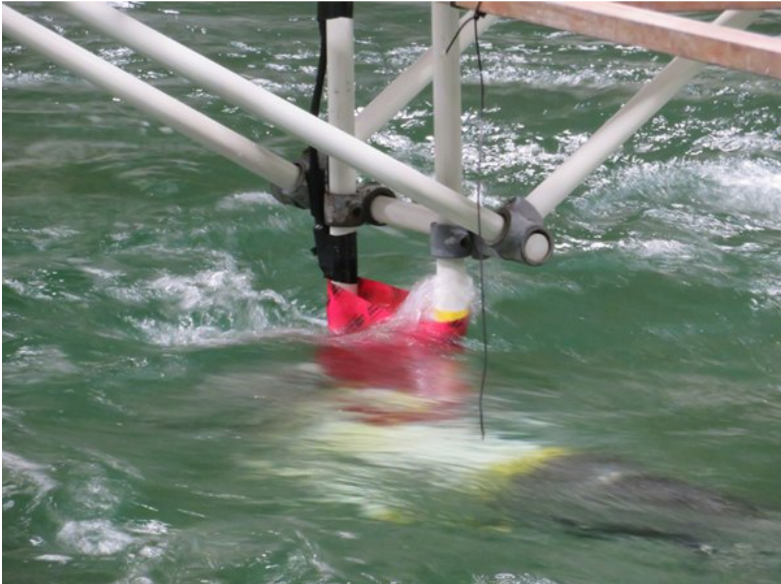
Figure 6: MicroRider in high flow (discharge 100%).
