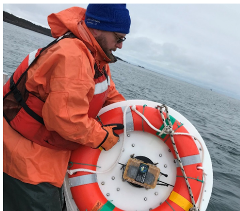
Left: Drifter sea trials to measure and map turbulence. Grand Passage, NS.
