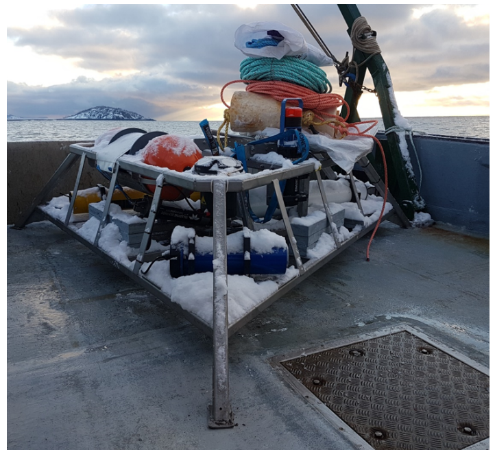
Above: FORCE FAST-3 platform, used for the deployment of the hydro-acoustic technology to conduct the stationary data collection surveys.
