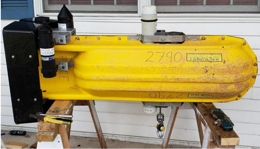
Figure 2.1.2. Prior to deployment at the Fundy Ocean Research Center for Energy (FORCE) test site VR2W-69kHz and HR2-180kHz receivers were mounted to Streamlined Subsurface Buoys (SUB) buoys by Dr. Brian Sanderson at Acadia University.
