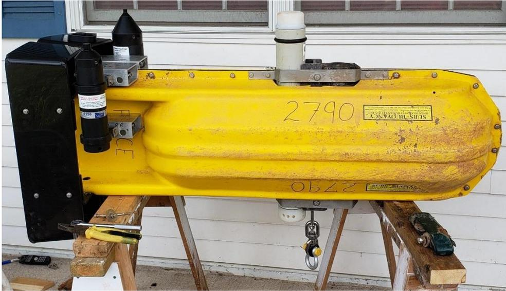
Figure 2. Prior to deployment at the Fundy Ocean Research Center for Energy test site VR2W-69kHz and HR2-180kHz receivers were mounted to Streamlined Subsurface Buoy buoys by Dr. Brian Sanderson at Acadia University.
