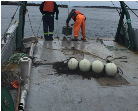
Figure A-15. Excessive biofouling (seaweed) on surface float line.
