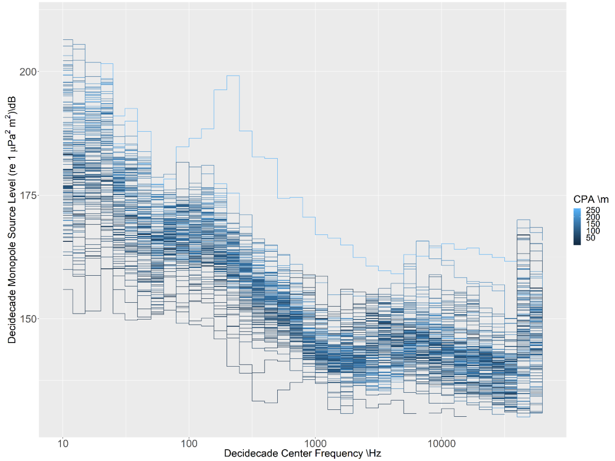
Figure D-7. Monopole Source Level for the ferry Margaret's Justice computed using the propagation loss shown in Figure D-1. The colour of each line indicates the distance to the closest point of approach distance.
