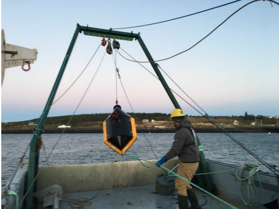
Figure A-13. High Flow Mooring being retrieved using the A-frame on the stern of the Nova Endeavour
