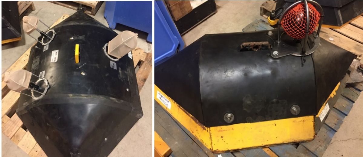
Figure A-2. High flow mooring with (left) an AMAR and three visible hydrophones (channels 1–3, channel 4 inside the shield) and (right) the Projector.
