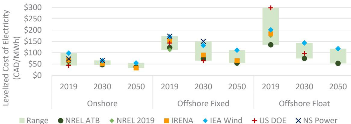
Figure 7 – Levelized cost of electricity from wind power
