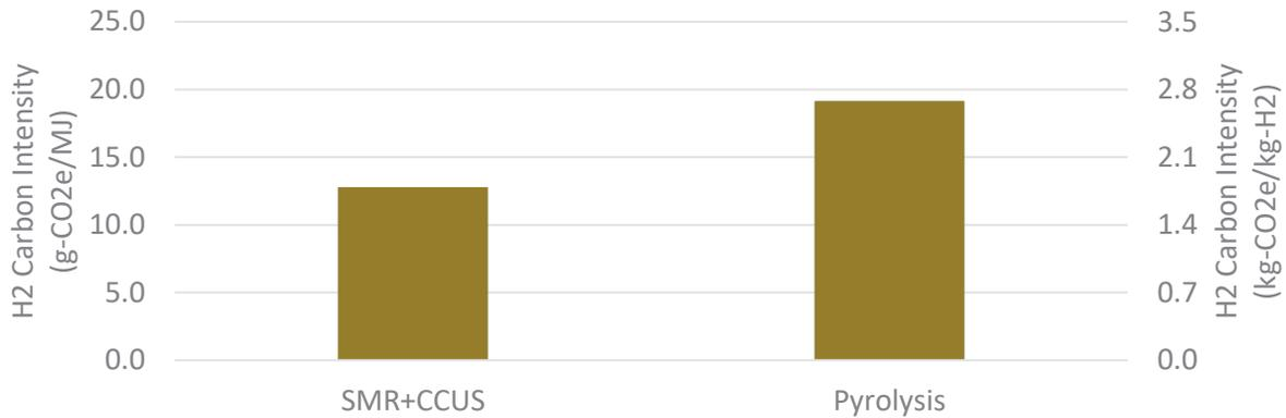
Figure 13 – Hydrogen carbon intensity – SMR + CCCUS and Pyrolysis
