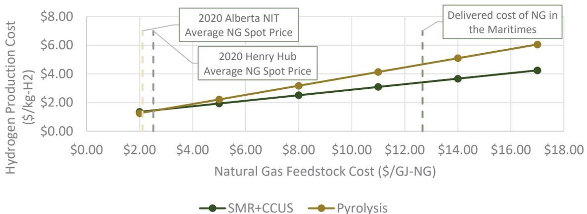
Figure 12 – Hydrogen production cost – SMR+CCUS and pyrolysis
