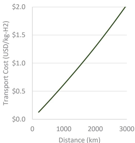
Figure 20 – Predicted pipeline hydrogen transport cost by distance overland<sup>45</sup>
