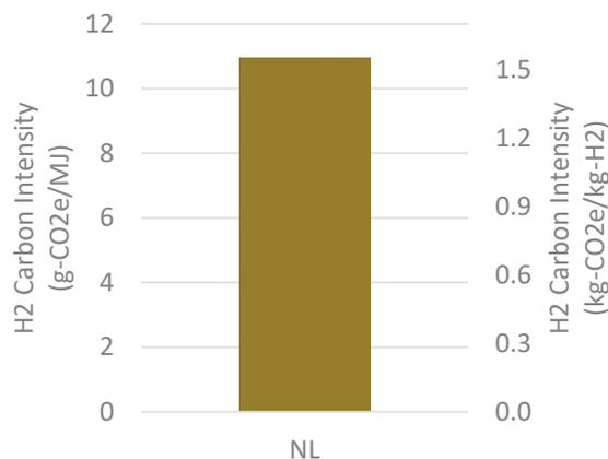
Figure 6 – Hydrogen carbon intensity – grid electricity electrolysis
