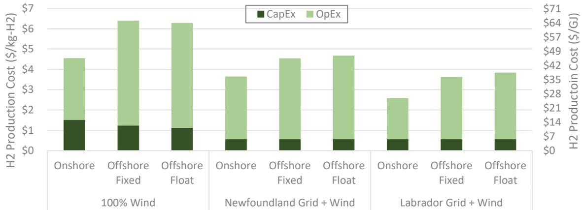
Figure 10 – Hydrogen production cost – wind power electrolysis
