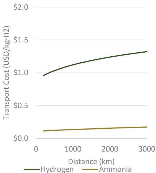
Figure 19 – Predicted hydrogen transport cost by shipping by storage method and distance<sup>45</sup>
