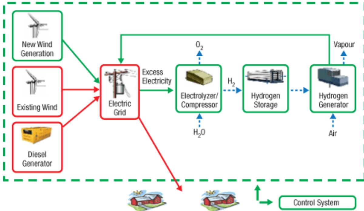
Figure 4 – Ramea Island Wind-Hydrogen-Diesel Project configuration<sup>14</sup>
