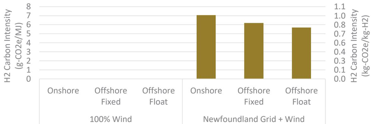
Figure 11 – Hydrogen carbon intensity – wind power electrolysis
