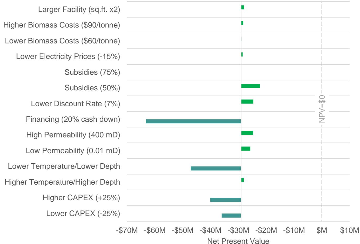
A sensitivity analysis was conducted on the optimal greenhouse scenario by independently varying facility size, energy costs, financial parameters, geological inputs, and geothermal system costs. The horizontal bars represent the impact of changing isolated variables on the overall NPV.
