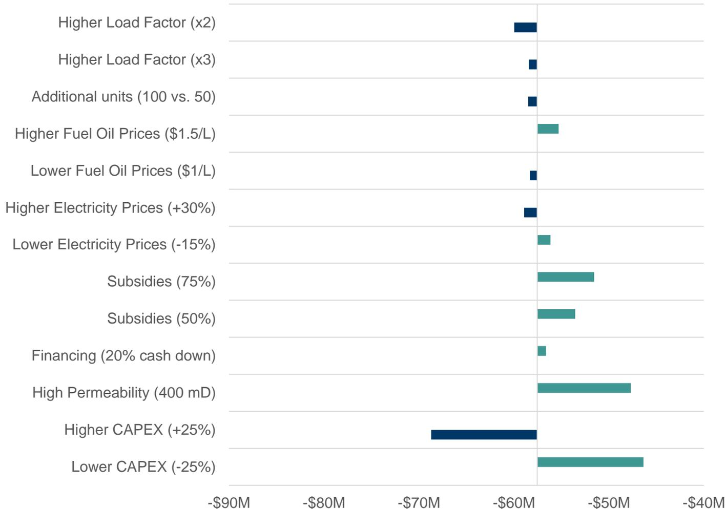
A sensitivity analysis was conducted on the optimal district heating scenario by independently varying the number of housing and business units, the overall heating load profile of the units and community center, energy costs, financial parameters, geological inputs, and geothermal system costs.
