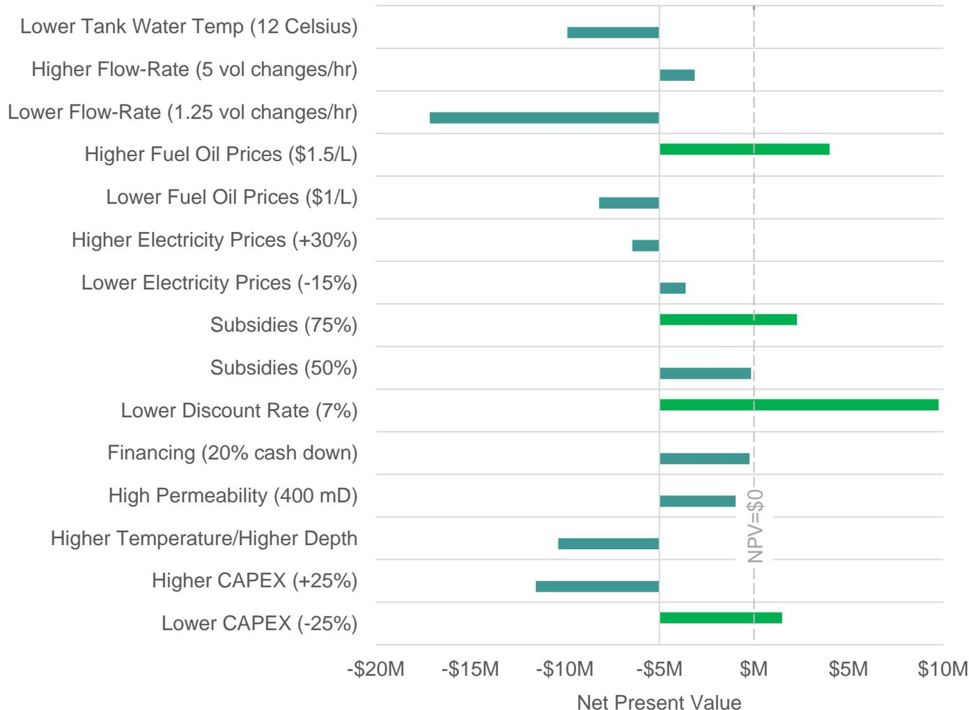
A sensitivity analysis was conducted on the optimal aquaculture scenario by independently varying water tank temperature, energy costs, financial parameters, geological inputs, and geothermal system costs.
