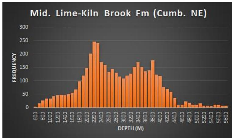
Distribution plots of the depth (left graph) and temperature (right graph) expected in the northeastern part of the Cumberland sub-basin for the Lime-Kiln Brook Formation. Each data point corresponds to a geographic cell on the map.
