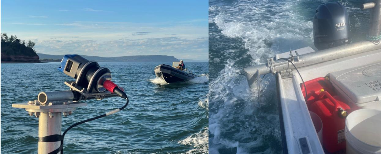
*Figure 2.1.10: Pole-mounted Gemini on research vessel Puffin*
